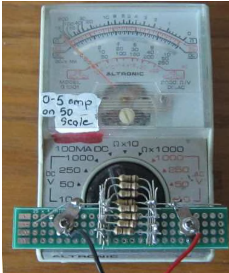
Turning an old meter into a valuable 0-5Amp meter
