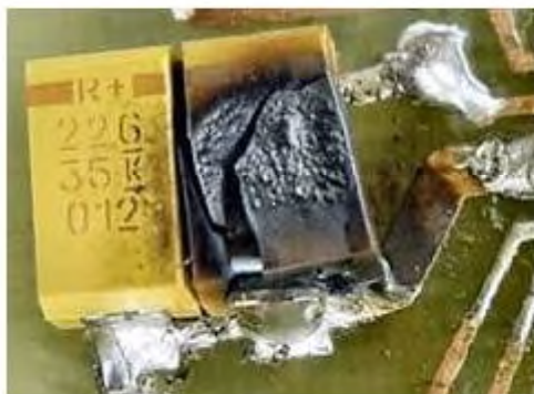
tantalum capacitors can "go up in smoke"
