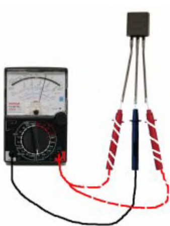
This is an NPN transistor The black probe is the BASE
