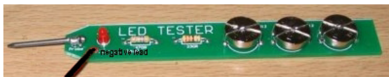
LED TESTER - tests LEDs See the project: HERE
